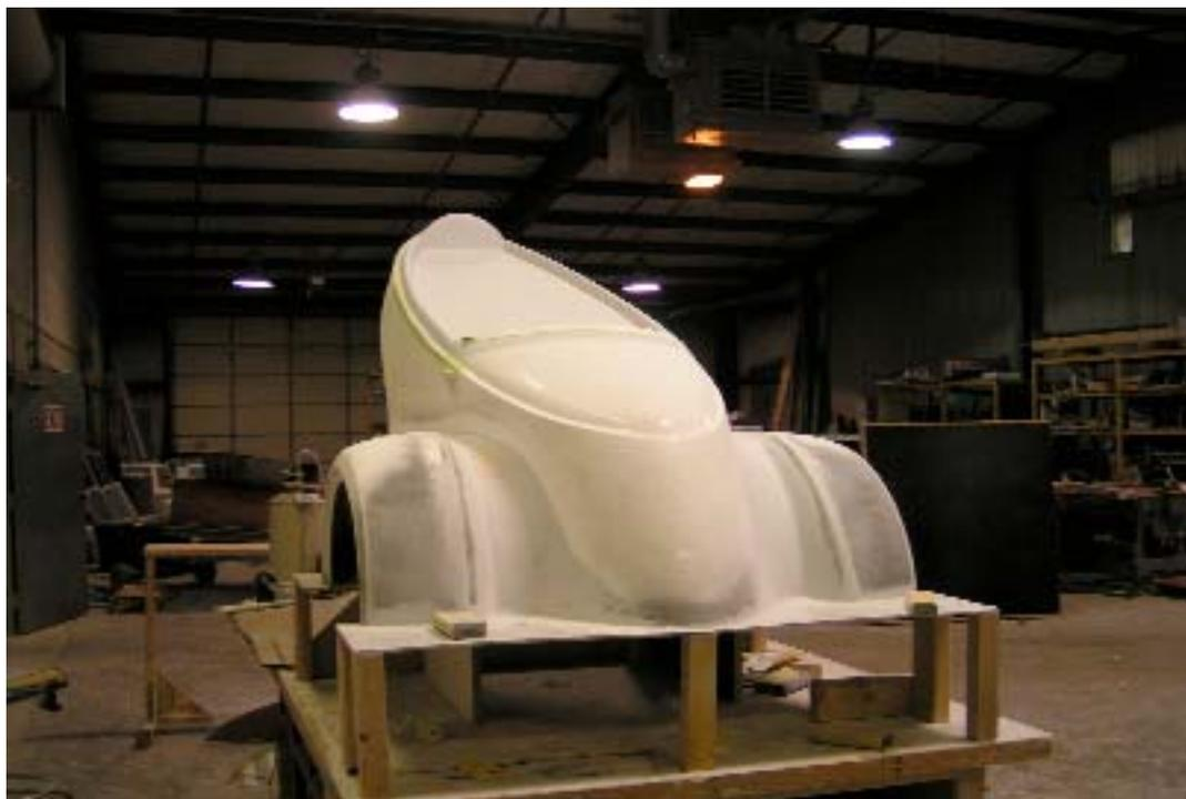
**The Fenders and Fairing shell were bonded together, and then sculped to blend into one piece. Once this part was finished, we made a lower portion in front to be a storage compartment. This part would also locate the Fairing to the front axle and form inner fenders that would strengthen the structure.**
