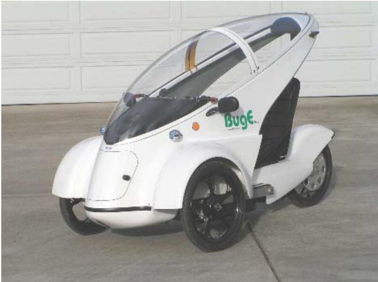
**The prototype has proven itself to be reliable and exceeds our expectations. It has a top speed of over 50 mph and a 30 mile range at 30 mph.**
