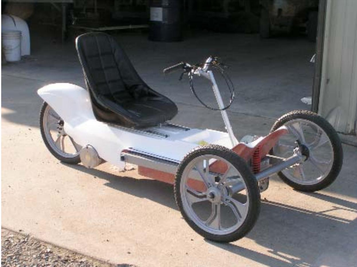
**The motor was fitted to the chassis, and connected to the rear wheel with a chain. The remaining space under the Seat pan houses the controller and battery chargers, and other electrical parts. This enables all the parts to be located together to simplify the wiring and servicing.**
