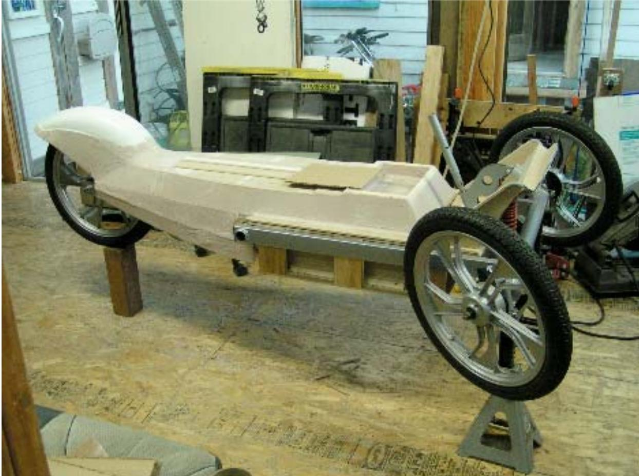
**The Seat Pan was designed to tilt up for access to the motor and electrical parts underneath, and included a small tray in front of the seat. It also comprised the rear fender as well**
