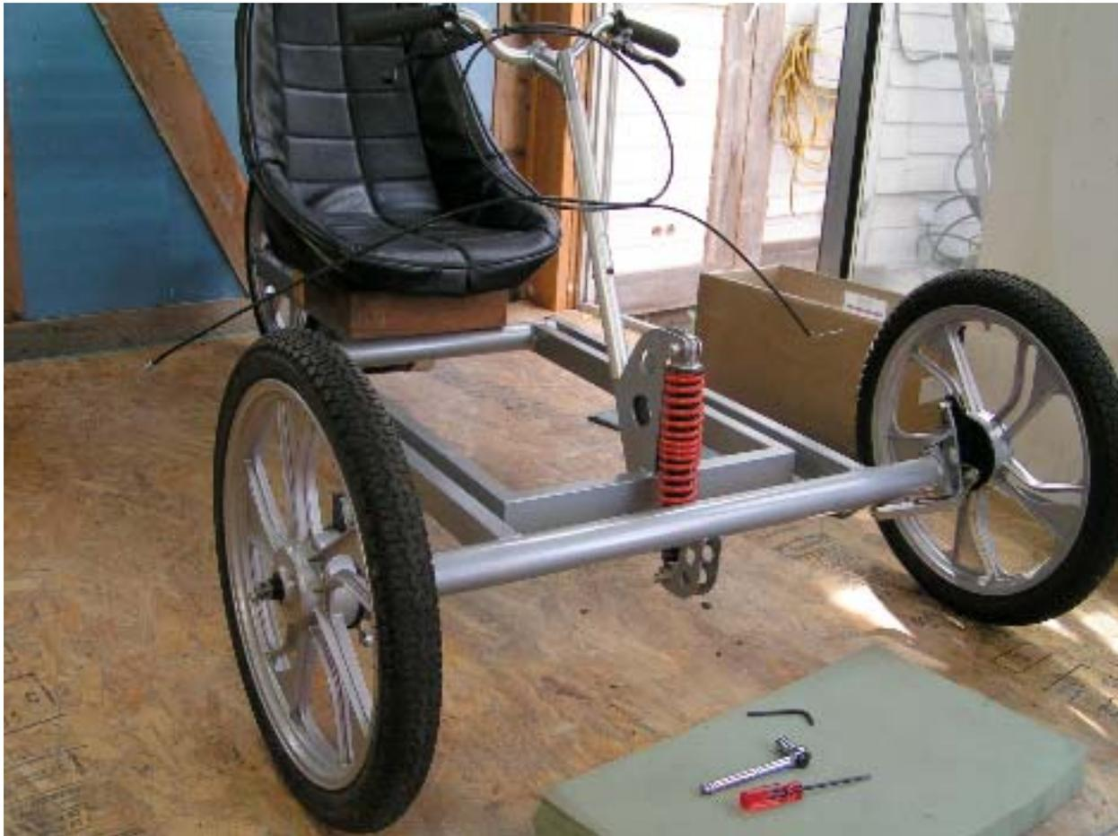
**The “cyclecar” layout of two wheels in front, one in back is based on the obvious fact that it is the more stable arrangement of wheels, providing two wheels for steering control and brakes.**
