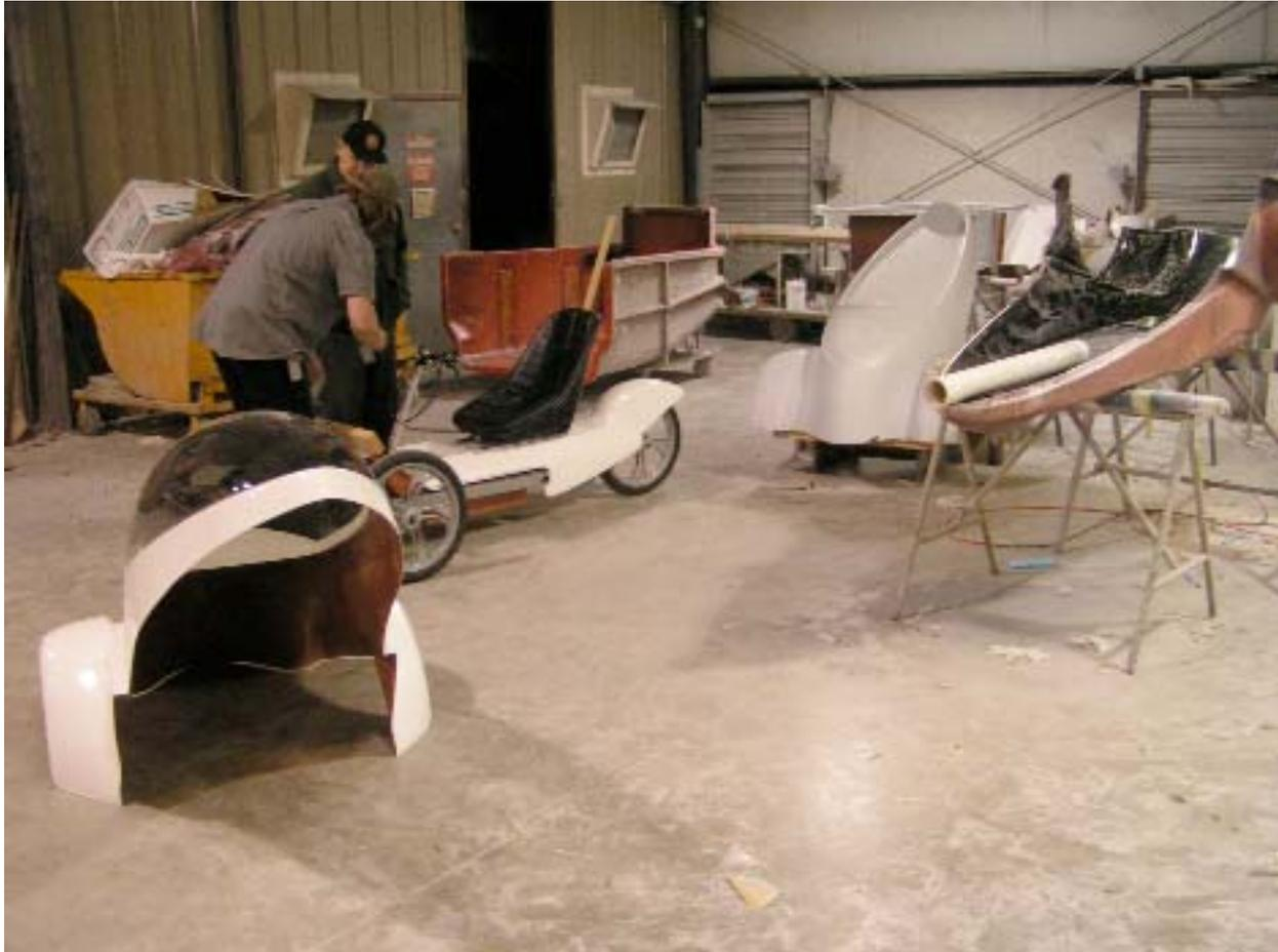
**Here you can see the grey Fairing plug, the Fairing mold upside down to the right, one of the Fairing parts, and the Chassis with the Seat Pan on it.**
