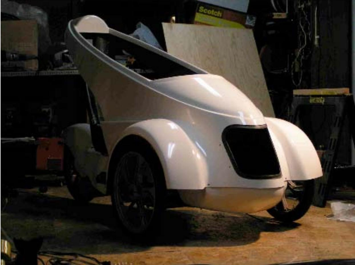
Finally the lower portion is bonded to the Faring to complete it. A hole is cut in the front to provide storage access and a door will cover the opening of course.
